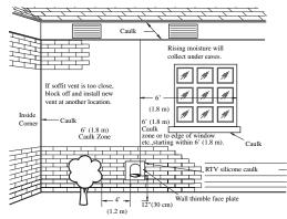
**A**WARNING: Moisture in the flue gas will condense as it leaves the vent terminal. In cold weather this condensate can freeze on the exterior wall, under the eaves and on surrounding objects. Some discoloration on the exterior of the building is to be expected. However, improper location or installation can result in severe damage to the structure or exterior finish of the building.
